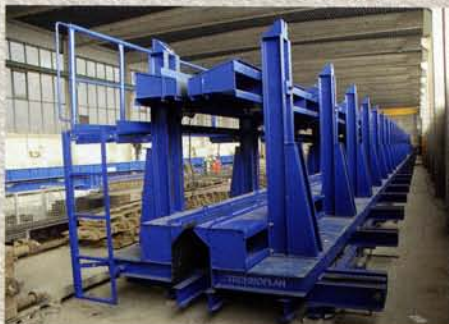
Hydraulic girder formwork system with continuously variable adjustment of both the height and inclination of the upper chord. Equipped with self-locking hydraulics, vibration plant and radio remote control.
