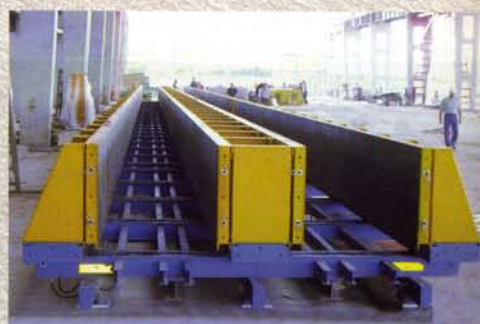
Hydraulic column formwork with adjustable steel formwork wall elements. Equipped with self-locking hydraulics, vibration plant and radio remote control.
