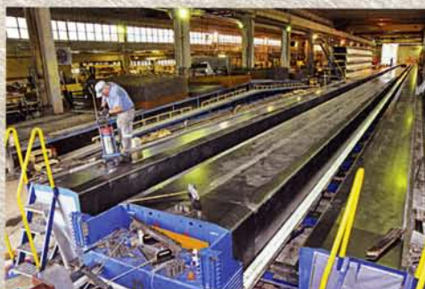
Stiffened hydraulic double T formwork providing 5000 kN tensioning force. Equipped with self-locking hydraulics, vibration plant and radio remote control.
